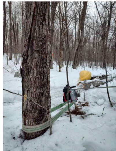
I typically skid two or three logs and then move anchor points.
